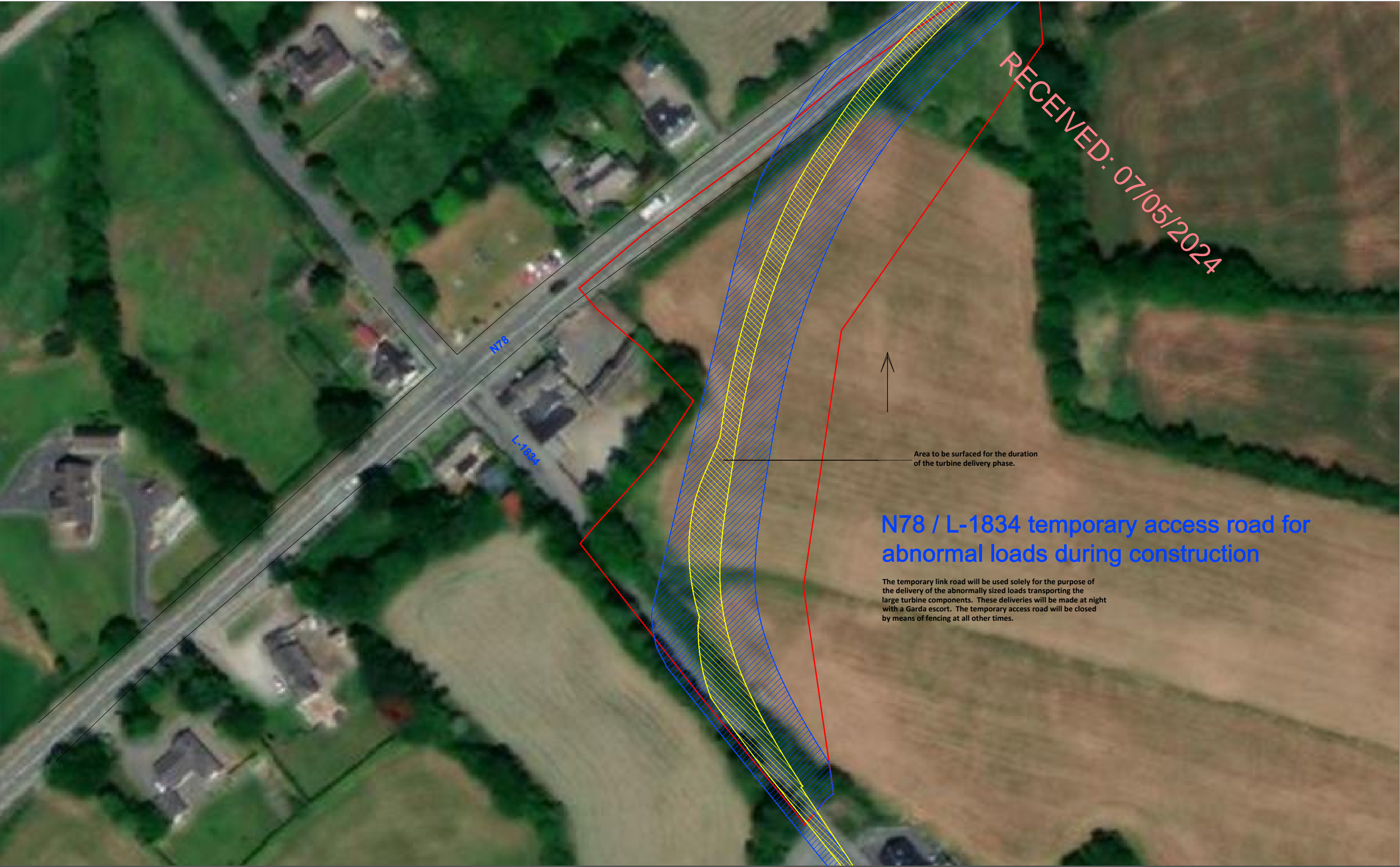
Figure 15-8 Location 5 - N78 / L-1834, proposed temporary access road for abnormally sized loads during construction phase
