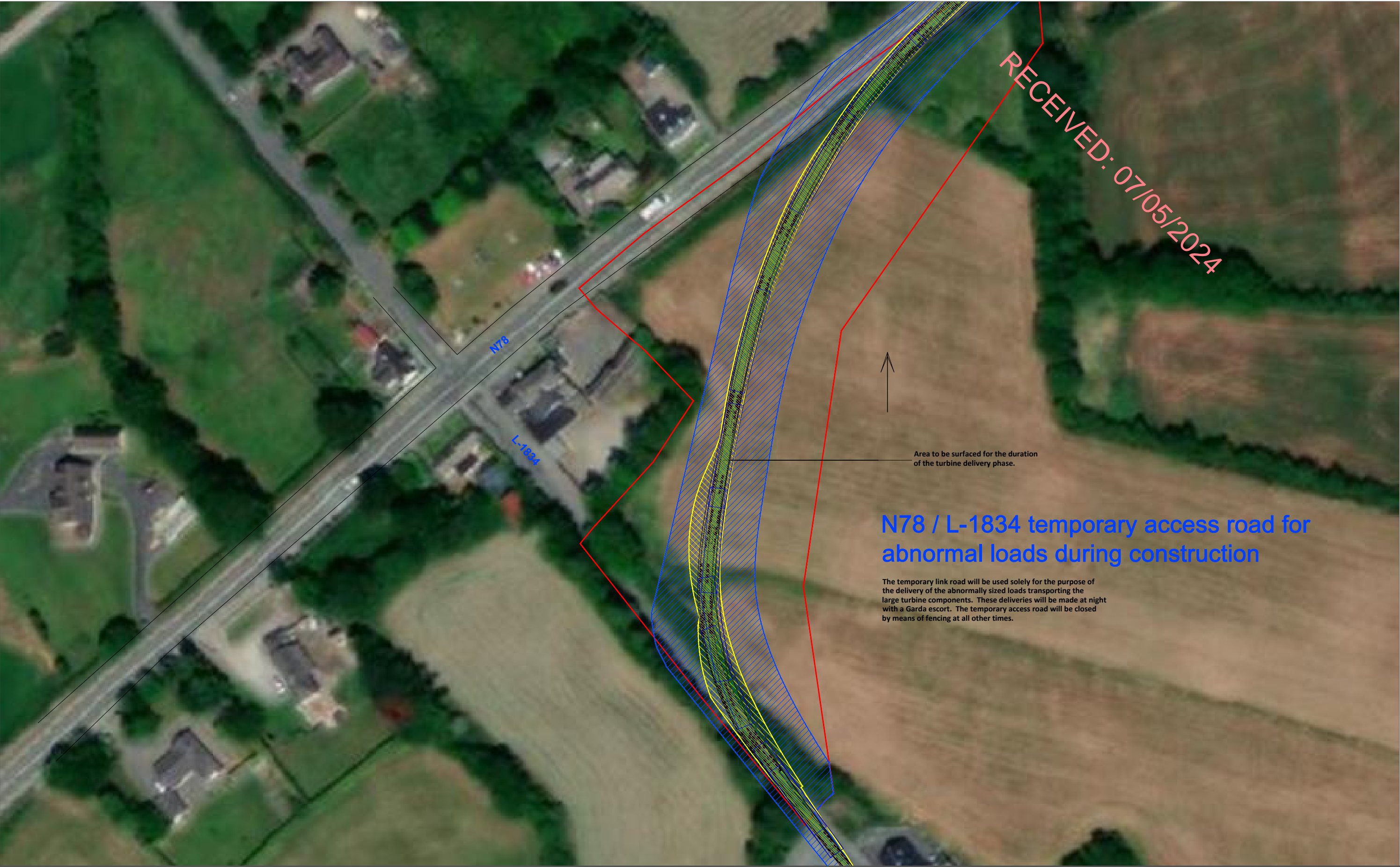
Figure 15-10 Location 5 - N78 / L-1834, proposed temporary access road for abnormally sized loads - tower extended artic
